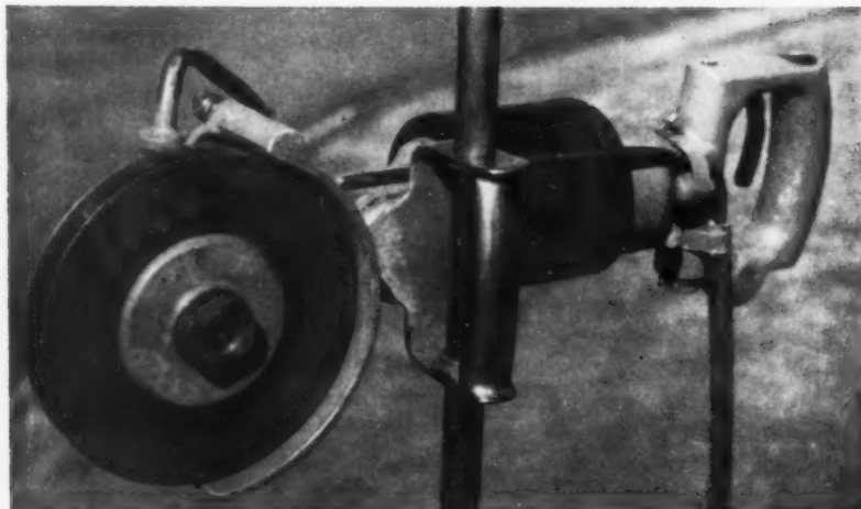
The "St. Clair Sampler" is equipped with two diamond saws and is shown here mounted on the support rod.
